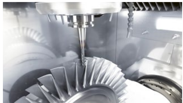
Dynamic positioning: Machining of aircraft turbine element
