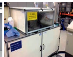
Impulse pressure test stand up to 4000 bar.
