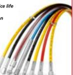
**70 MPa (DN 6)** - Inner tube of polyamide (PA), 2 spiral layers of high tensile steel wire, 2 open spiral synthetic fibre, outer sheath of polyurethane (PUR)
